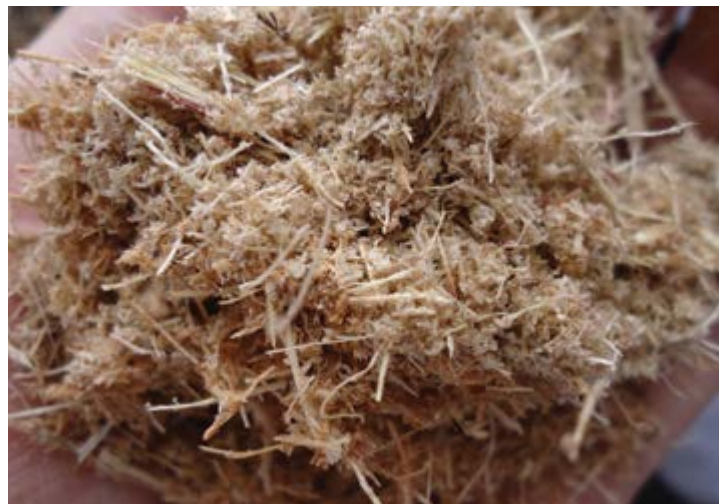
Sugarcane bagasse used in cogeneration power plant
