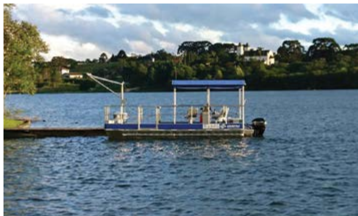
Platform equipped with devices to measure several quality factors in the Passaúna dam, in the Paraná state
